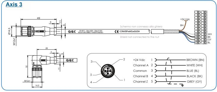
Don't connect or disconnect the circular connector or the terminal block in presence of voltage. The connection in presence of voltage may result in electrical discharges that are potentially harmful to the equipment, the connectors and the user..
