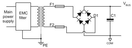
In order to reduce the influence of EMI disturbances, it is recommended the use of our AC/DC converters with intergrated filters AL1120 or AL2620, or as an alternative, of a specific network filter (like CORCOM 10AYO1 in case of three-phase supply, or CORCOM 10VT1 in case of single-phase supply).
