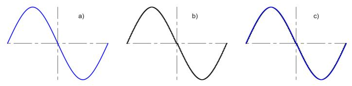
Profile of current to the motor: a) VectorStep with stepless technology b) Traditional microstep drive c) Comparison of profiles
