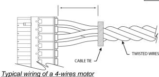
In case of twisted wires, fix the twist with a cable tie e let the cables free for the minimum distance you can see in the table.
