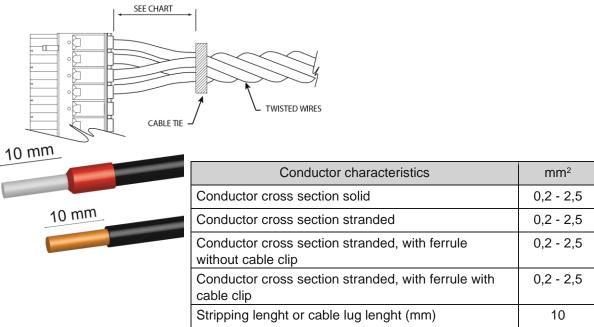
In case of twisted wires, fix the twist with a cable tie e let the cables free for the minimum distance you can see in the table.
