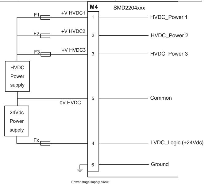
The configuration of the input circuit independently supplies the control stage with respect to the power stage.
