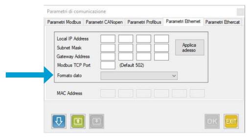
It is possible to choose between "Intel (Little Endian)" 32 bit mode (first read/write the lowest 16 bit word then the highest 16 bit word) or (Motorola (Big Endian)" 32 bit mode (first read/write the highest 16 bit word then the lowest 16 bit word).
