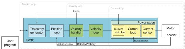
Servo-mode function is realized by using a stepper motor with an encoder feedback, in order to obtain a position feedback. The encoder doesn't only control the motor position, but, thanks to the EVSC, becomes an electronic collector which permits the drive to react real-time to load variations.
