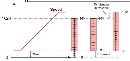
As shown above, it is possible to act on the offset register and on the multiplication and division constant in order to shift the analog register, with the purpose to let the value 0 coincide to the minimum reference value (Offset) and to compress or dilate the scale with the purpose to let the value 1024 coincide to the maximum reference value (Rmulanainp and Rdivanainp).
