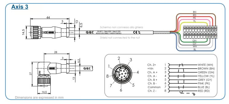
Don't connect or disconnect the circular connector or the terminal block in presence of voltage.
