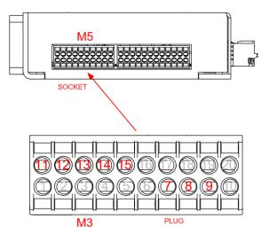
Caution!!! The inputs and the outputs 0-7 share the same pinout. In order to avoid damages to the connected devices, never active an output when the same pin is used as an input.
