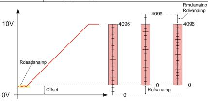
As shown above, it is possible: to create a dead band (yellow zone) in order to eliminate disturbances of the reference in proximity of the minimum value; to shift the analog register in order to let the 0 value coincide with the reference minimum value (Offset); to compress or to expand the scale in order to let the value 4096 (full scale) coincide with the maximum reference value (Rmulanainp and Rdivanainp). In this case, the value of the analog register will be:
