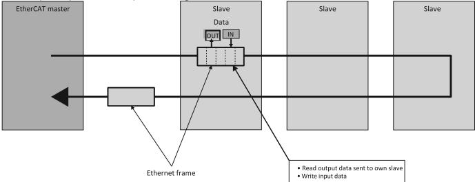
The EtherCAT protocol transports data directly within a standard Ethernet frame. Data is communicated between master and slaves in the form of process data objects (PDOs). Each PDO has an address to one particular slave or multiple slaves, and this "data and address"
