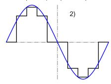
Difference between the profile of current of a traditional drive and a VectoStep drive at full step (1) and at half step (2)
