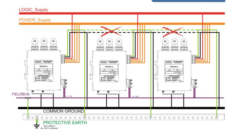
CAUTION !!! A wrong positioning, connection, shielding or grounding of the drives or devices connected to the drives, may cause electromagnetic disturbances.
