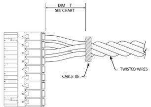
In case of twisted wires, fix the twist with a cable tie e let the cables free for the minimum distance you can see in the table.
