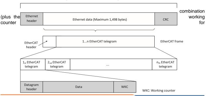
validation) makes up an EtherCAT telegram. If an Ethernet frame is compared to a "train," an EtherCAT telegram would be a "compartment."
