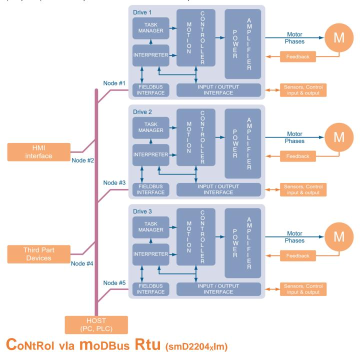
Modbus is a serial communication procol created by Modicon in 1979, in order to put into communication their PLC. It in fact became an industrial standard since 1979, MODBUS permits million automation devices to communicate between each other, by using a request/response type communication, and services defined by function codes. The main reasons for such a wide utilisation of Modbus compared to other protocols are the following:
