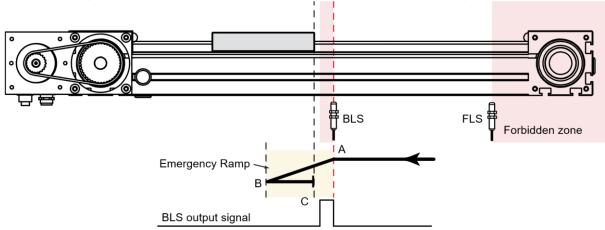
As shown in the illustration above, the drive blocks the movement after the intervention of the back limit switch (point A), braking the motor in emergency ramp until it stops in the point B.
