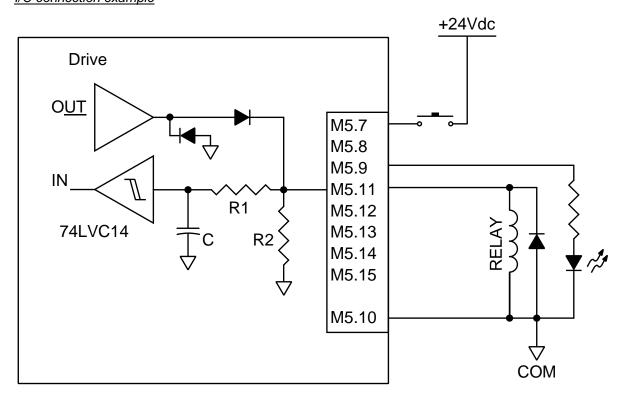
©Caution!!! In case you need to drive inductive loads (like relays, electro-valves, etc.) connect a flyback diode (1A @1000V) in parallel to the load.
